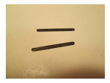
Drill 0.021" (#75 bit) holes in the levers as shown in the diagram below.
